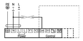
Power supply must not be connected to the signal terminals!
