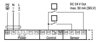
Switching contact requirements: The switching contact must be able to switch a current of 10 mA at 24 V accurately.
