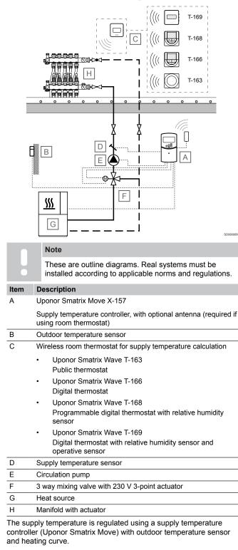
Connected to the supply temperature controller is the heat source, circulation pump, supply temperature sensor, and 3 way mixing valve.
