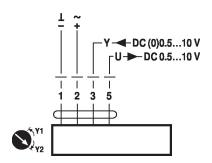
Override control (frost protection circuit)
